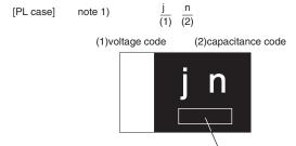
manufacture code note 2) voltage code and capacitance code are variable with parts number
